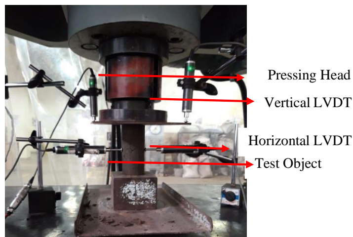
Figure 4. The position of the test object for compressive strength
