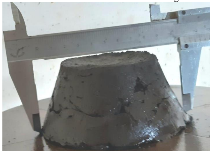
Figure 5. Flow of fresh geopolymer mortar
